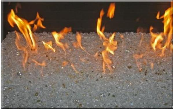
Now turn on the natural gas supply and light the burner with a safety lighter. Check to see that the flame is centered and going up (not lapping on the back wall; this will cause soot and will not look good). \* You can turn the pipes on your natural gas burner to have the holes facing down and forward. This will change the flame pattern. Once your flame is how you like, it's ready for glass.
