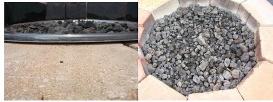
3) **IMPORTANT:** Do not cover blowout box with lava rock- leave open. Do not allow any rock to touch the thermocouple.
