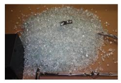
This picture shows the pilot in its proper position, No mounting is required the glass will support the pilot
